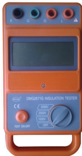
绝缘电阻测量 Insulation resistance tester
